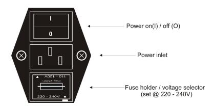
After connecting line power, the instrument can be switched on with the power switch on the rear of the instrument.
