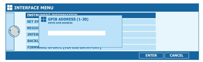
Enter the required GPIB address using the keypad, then select **ENTER** to save or **CANCEL** to abort.
