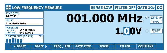
Pressing the **HF MEASURE** function key will set the unit to low frequency measurement mode. In this mode the instrument measures the frequency of the signal connected to the LF Measure Input. The maximum input frequency is 1.05 GHz, and the maximum input voltage is 1 V.
