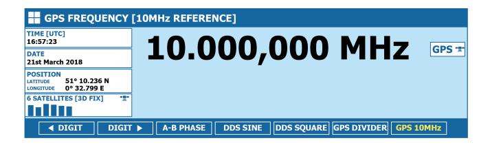
Pressing the GPS DIVIDER softkey when the unit is in LF SOURCE mode will set the 8700 to **GPS FREQUENCY [DIVIDER MODE]**. In this mode the output frequency can be varied in steps of 1, 2, 5 from 1 Hz to 5 MHz.
