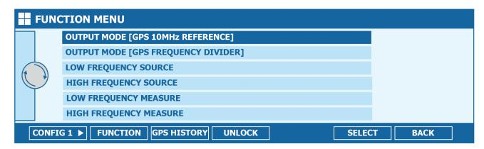
Select a menu item using the **DIGITAL DIAL** to select the corresponding function - the menu will close after function selection automatically
