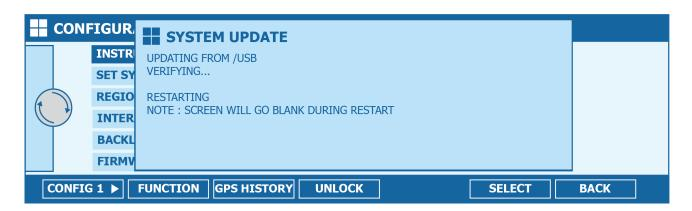
Once completed the user is prompted to **REMOVE** the **USB** drive - the system will then restart <u>after removal of the USB drive is detected</u>.
