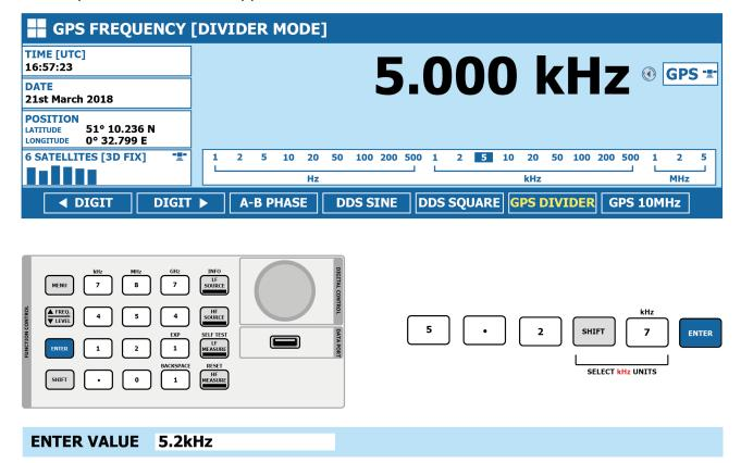
Pressing the DDS SQUARE softkey when the unit is in LF SOURCE mode will set the 8700 to LOW FREQUENCY SOURCE [DDS SQUARE WAVE]. In this mode the frequency can be varied from 10 Hz to 100 kHz in 1 Hz steps. The output is a fixed square wave with a peak to peak amplitude of 5V @ 1 MOhm.
