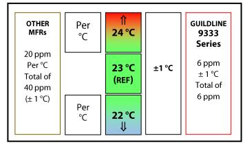
affects adjustment +5 °C at 20 ppm/°C and -5 °C at 20 ppm/°C)]. Applying a general rule of 4 to 1, this allows you to calibrate only instruments with a 0.1 % or larger specification.
