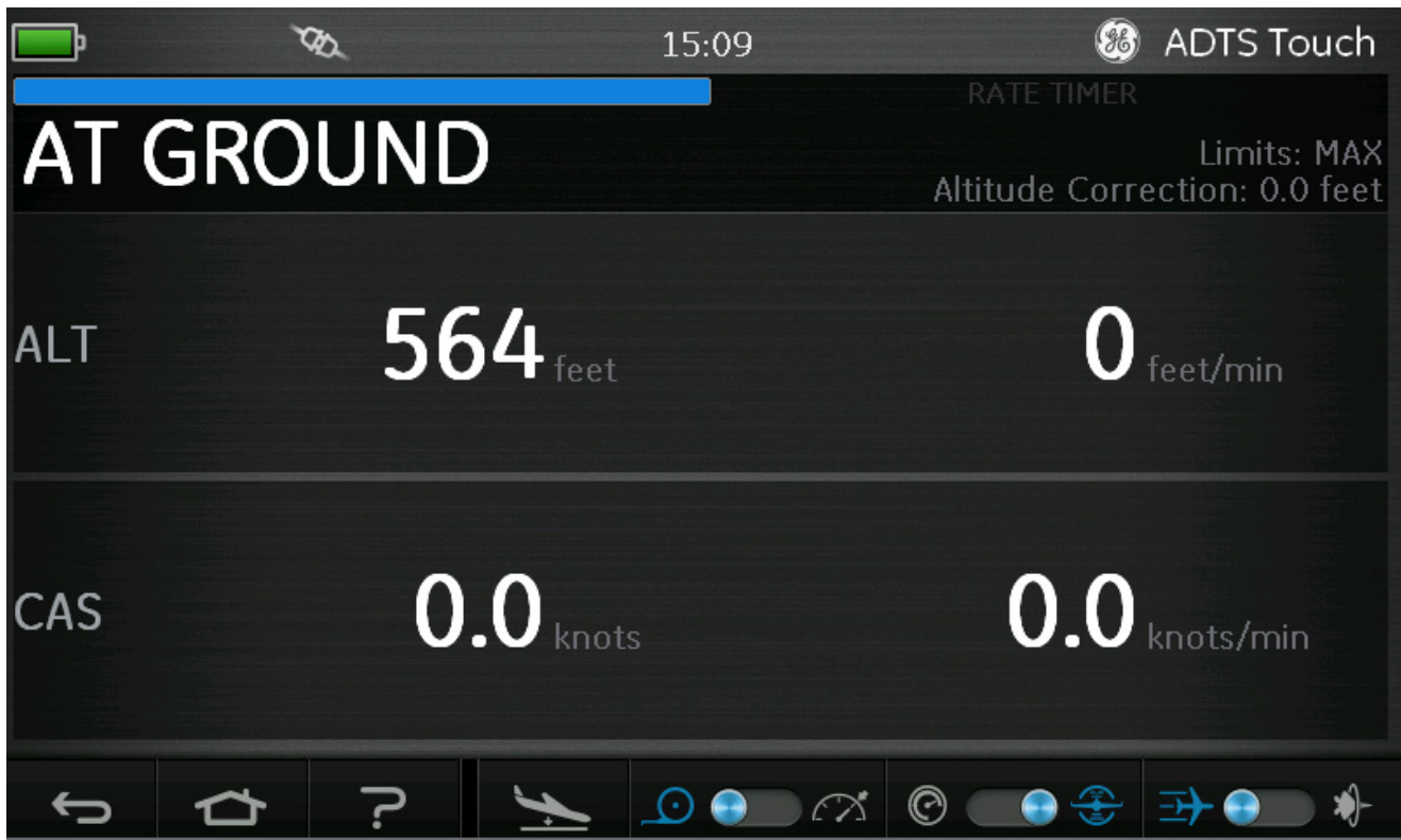
Figure 3-26:Go To Ground Complete
