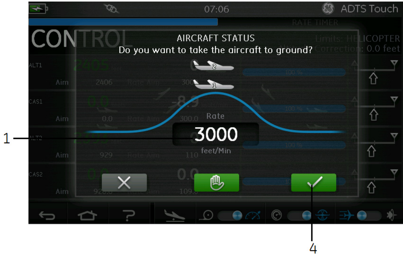
Figure 3-21: Start go to ground action - Multiple Channel
