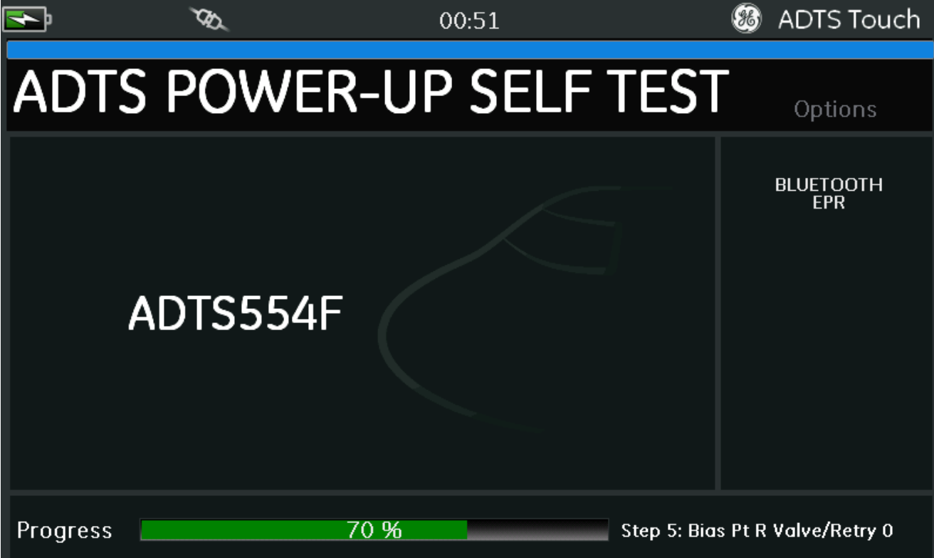
Figure 3-2: ADTS power-up self test screen with Bluetooth/EPR
