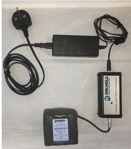
Figure 33 Spare Battery Charging
