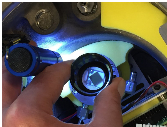
Figure 40 Checking the Mirror Surface
